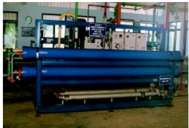
A plating effluent recycle plant at Sundaram Fasteners Ltd., Madurai, Tamil Nadu.
